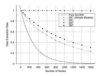
Figure 4: Experiment Set 1 - Single Sink: PureALOHA and  $SN^1$  (Simple Models) overlap. As the number of nodes increases, the DER decreases exponentially. With typical LoRaWAN settings  $(SN^3)$ and a typical DER > 0.9 requirement N = 120 nodes can be supported.
