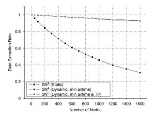
Figure 5: Experiment Set 2 – Dynamic Parameters: Lines for  $SN^4$  and  $SN^5$  overlap. When optimising transmission parameters for minimal airtime (or airtime and power) network capacity greatly improves. With minimised airtime ( $SN^4$ ) and DER > 0.9, well over N = 1600 nodes can be supported (compared to N = 120 nodes with static settings).
