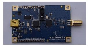
Figure 2: NetBlocks XRange RF module.
